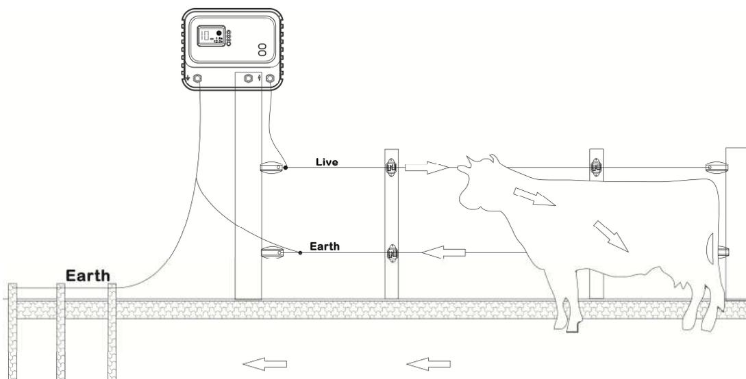
Final Step – Test voltage level at the end of the fence line with an electric fence tester. Voltage measurement should be at least 3000 volts.
