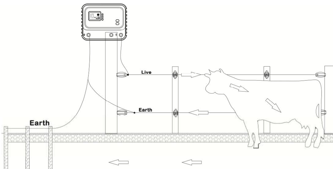
Final Step – Test voltage level at the end of the fence line with an electric fence tester. Voltage measurement should be at least 3000 volts.
