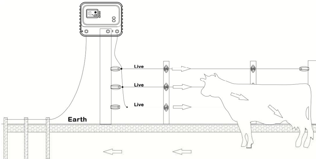
2. Pos./Neg. system: Where soils are not conductive e.g. dry, sandy, pumice soils as well as frozen soils or snow conditions, where an earth-return wire should be used in conjunction with the ground system – as per diagram. When the animal touches both a positive and a grounded wire, the animal will receive a shock.
